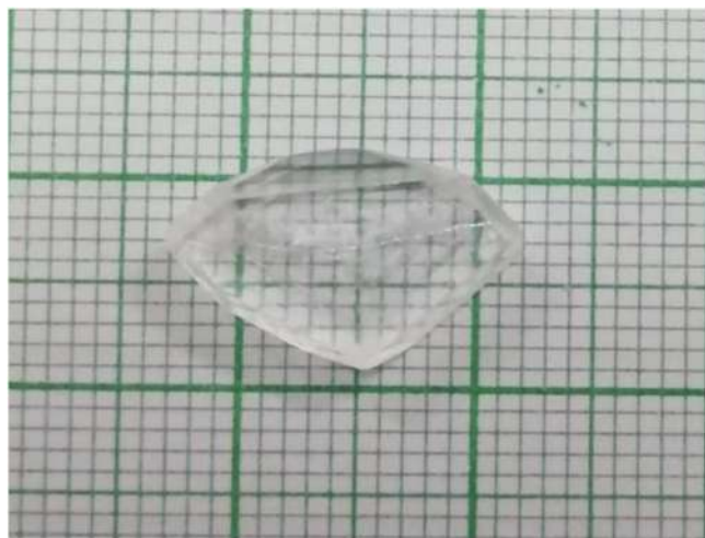
Fig. 1. As grown IMGA single crystal.
